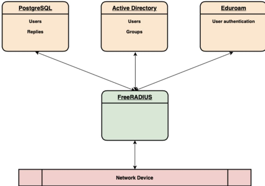
The network device will communicate with FreeRADIUS, which will determine if it should try to find the user in the local SQL database, do a lookup in AD or act like a proxy and forward the request to Eduroam. If we are going to use AD, we will first authorise the user with NTLM and in a second step use LDAP to lookup which groups the user belong to and based on that assign VLANs etc.
