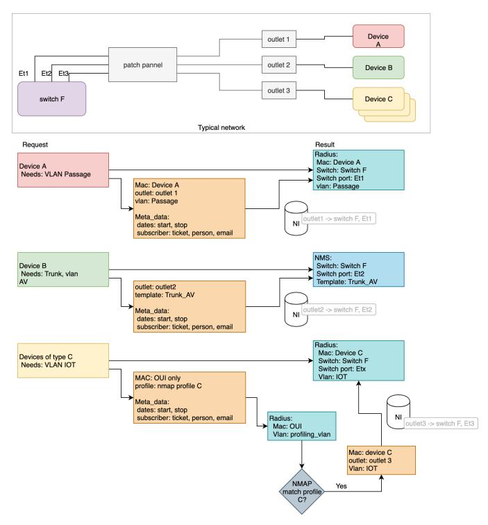
Except for dot1x are the client assignment today to based on the physical port in the access switch.
