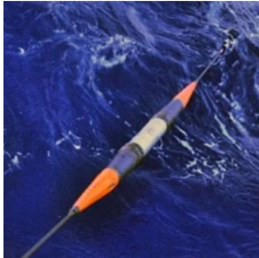
SMART cable sensor
